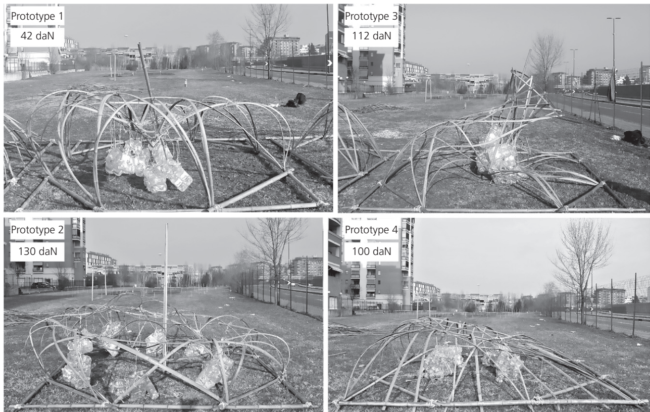
Figure 3. Prototypes at failure
