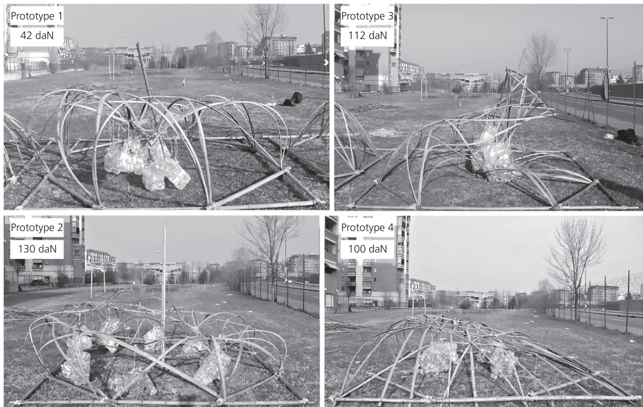
Figure 3. Prototypes at failure
