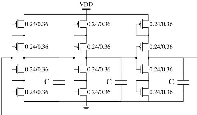
Fig. 2: Three stages starved Ring Oscillator (RO).
