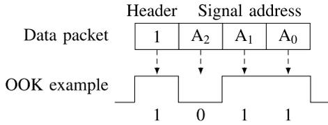
Fig. 4: Packet template and example of OOK modulation.
