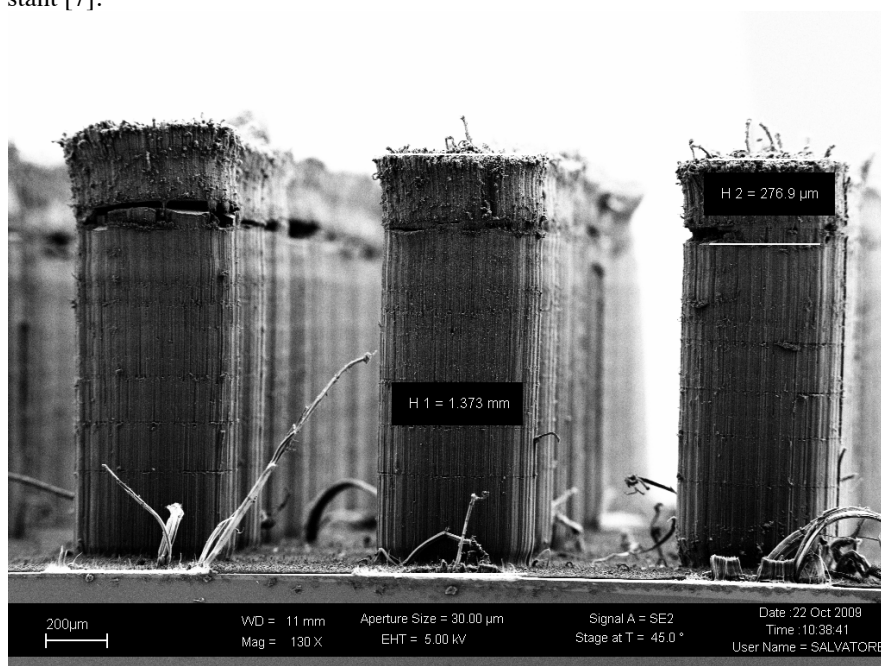
Fig. 6.9 Free standing vertically aligned multi wall carbon nanotube
