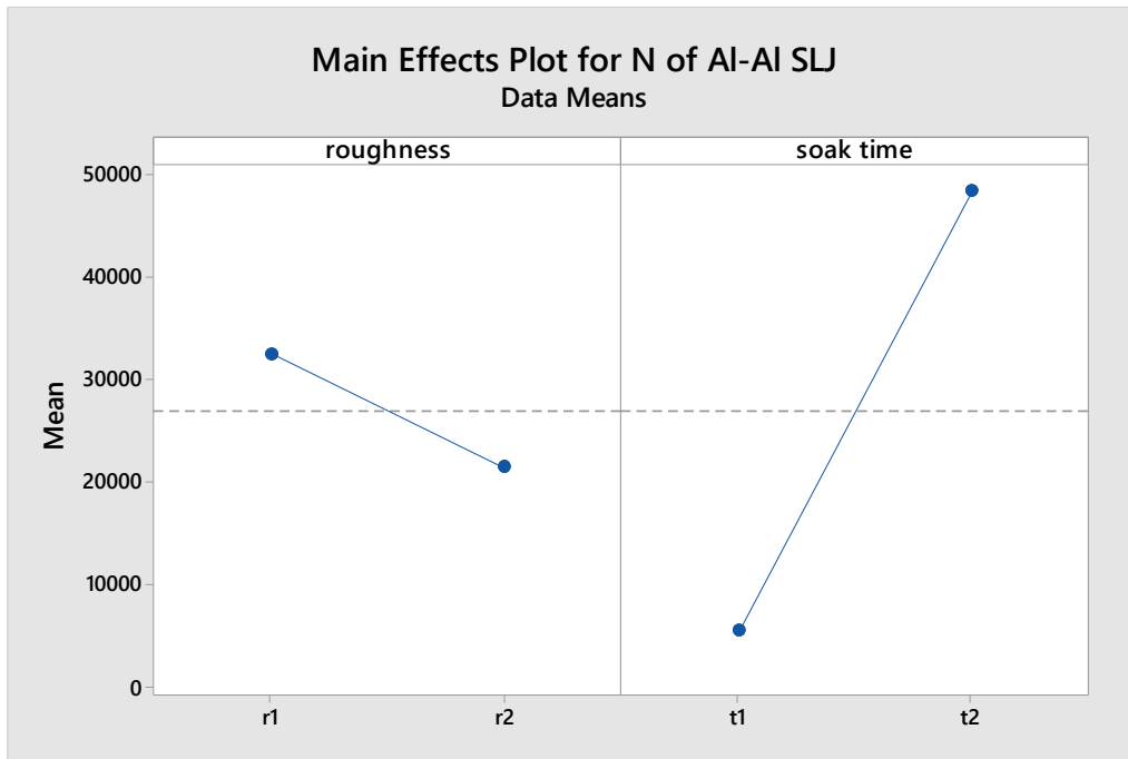
Figure 15. Main Effects Plot for Fatigue Life of Al-Al Joints under F_{alt} = 20\% of LTC.
