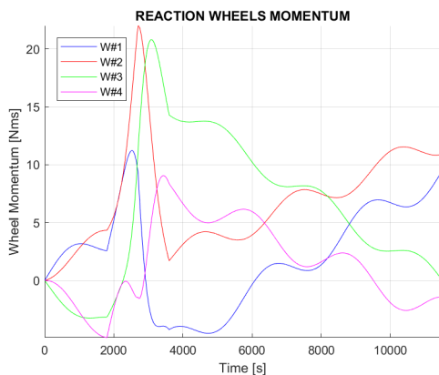
Fig. 7: CTA-SMC Reaction Wheels momentum.
