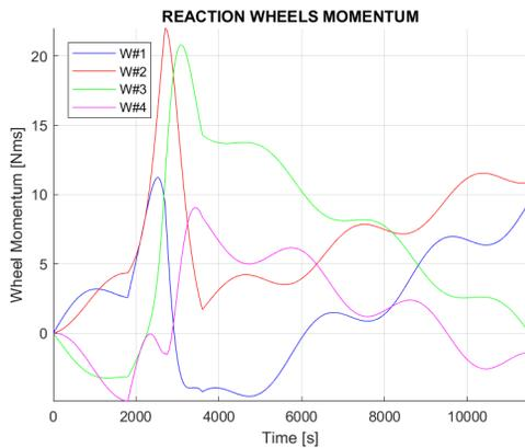
Fig. 7: CTA-SMC Reaction Wheels momentum.
