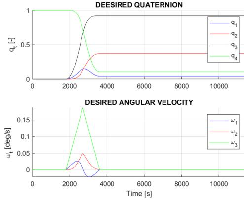
Fig. 1: Reference inertial quaternion and angular velocity.
