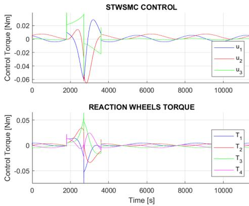
Fig. 3: STW-SMC control and Reaction Wheels torque.
