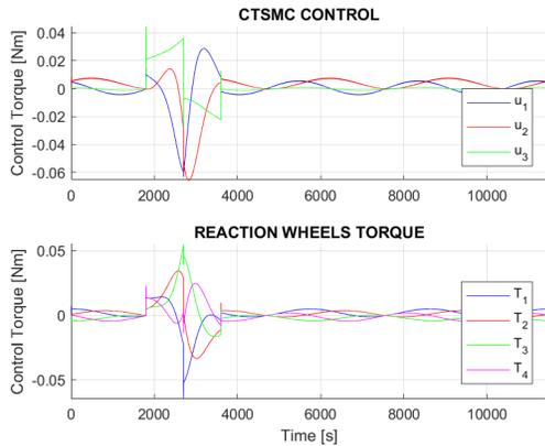
Fig. 6: CTA-SMC control and Reaction Wheels torque.
