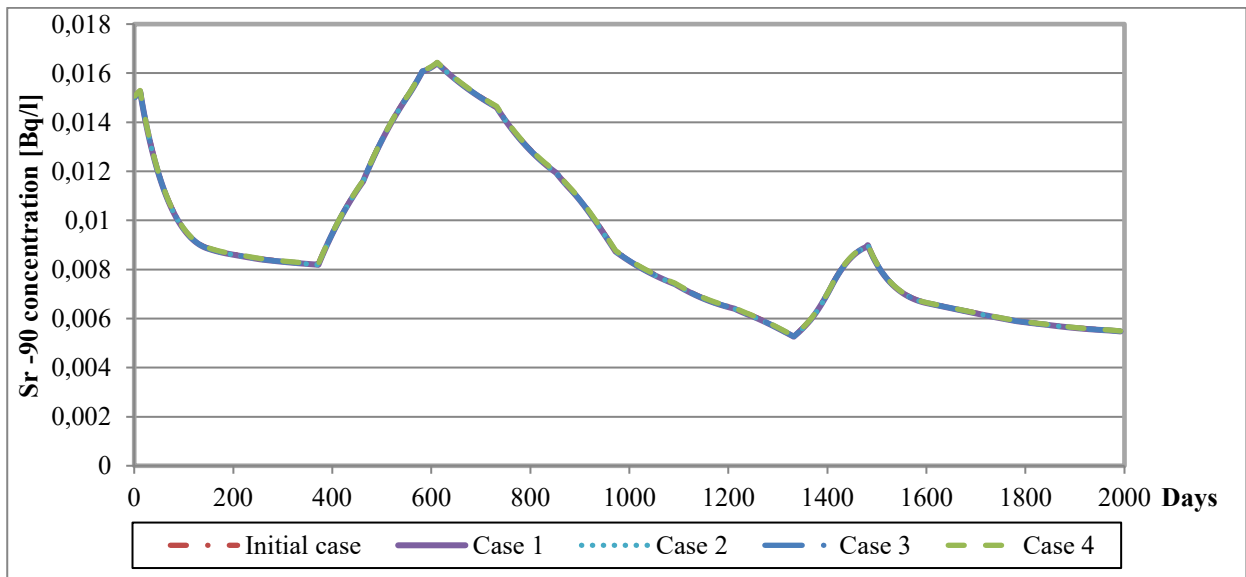
Figure 5 Sr-90 concentration in SP01 monitoring well for flow rates in Cavour channel equal to 14.67 \text{ m}^3/\text{s} (initial case), 7.33 \text{ m}^3/\text{s} (case 1), 1.47 \text{ m}^3/\text{s} (case 2), 44 \text{ m}^3/\text{s} (case 3), 146.67 \text{ m}^3/\text{s} (case 4).
