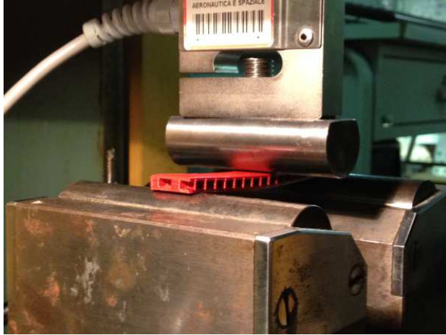
Figure 2: Specimen 1 during the three-point bending test.
