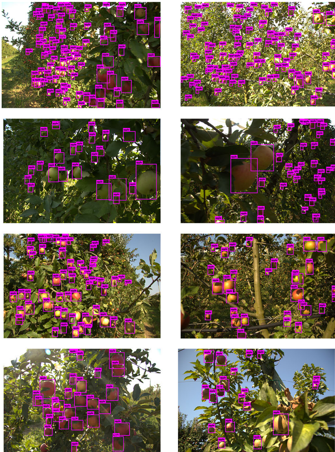
FIGURE 7. Qualitative results of some additional test images acquired from the same study site of the training data set. It is possible to notice how our custom version of YOLOv3-tiny is robust to different factors of variation [56] in how apples appear. Simultaneously handling variations in illumination, viewpoint, scale, occlusion, and background clutter is a challenging task that our system has to tackle in real-time with limited computational capabilities.
