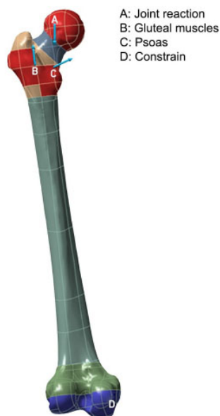
Fig. (1). Load and boundary conditions related to gait heel strike phase.
