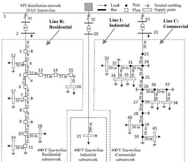
Figure 1. Cigré low voltage test grid [19]
