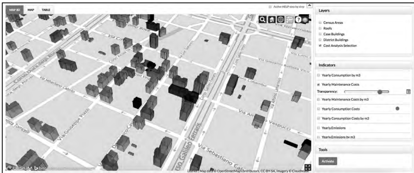
Figure 4 - Visualisation of the maintenance costs for some of the considered buildings
