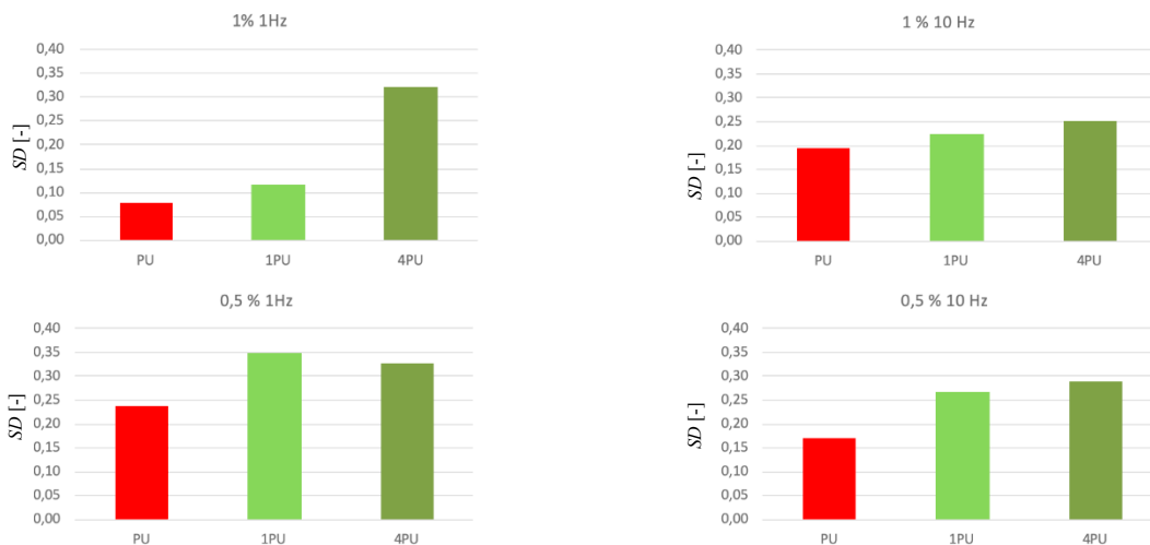
Fig. 4. Stiffness degradation in different strain and frequency conditions for different number of PU coating layers.
