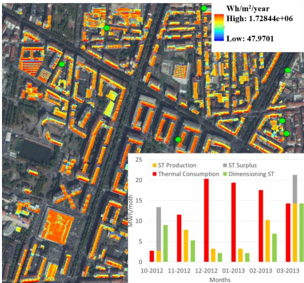
Figure 15. Solar resource, energy production and potential energy productivity
