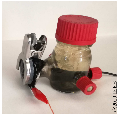
Figure 2.12: Picture of the Single Chamber Microbial Fuel Cell: a Pyrex® bottle of 0.125 L volume equipped with the air-breathing cathode on the opening on the left side, the anode connected through the small opening on the right side and the big opening on the top for positioning the sample electrode. [28]
