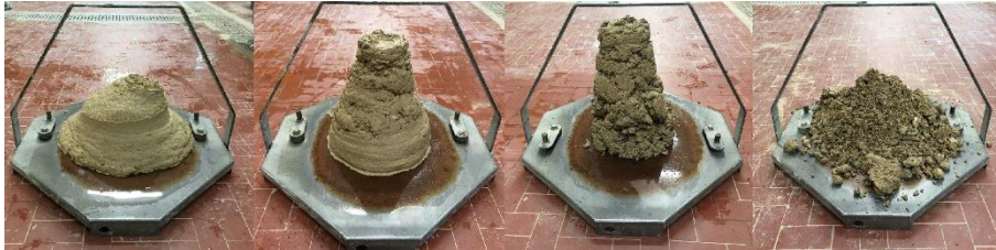
Fig 2 Slump test on the a morenic soil at different times from production (from left: production, 1, 3 and 7 days). It is possible to see the change of behavior with time.
