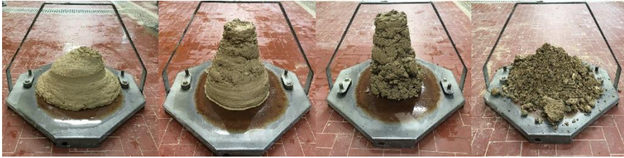
Fig 2 Slump test on the a morenic soil at different times from production (from left: production, 1, 3 and 7 days). It is possible to see the change of behavior with time.
