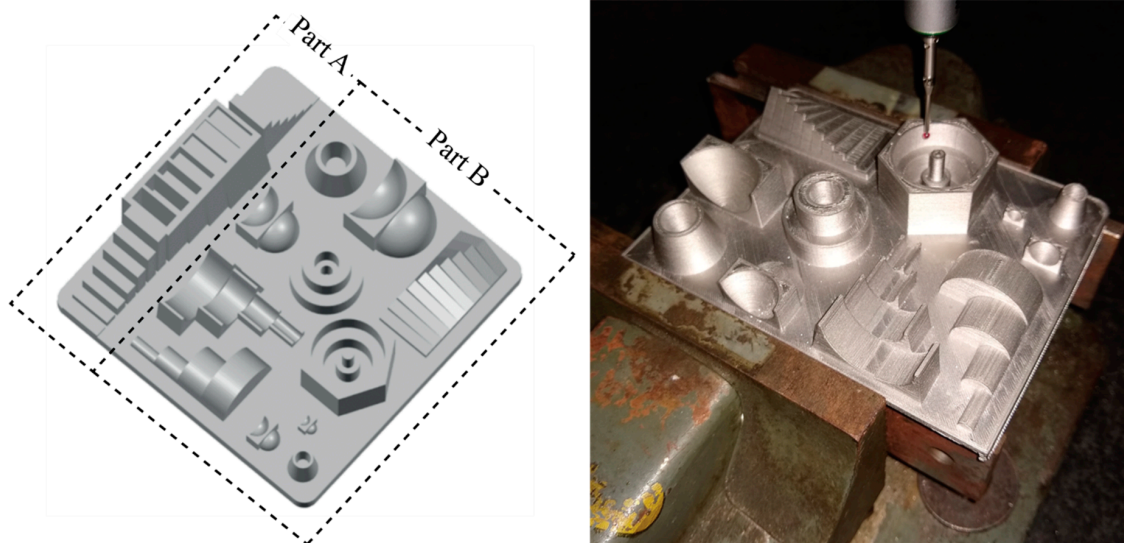
Figure 5. Geometry of the reference artefact [16] for the evaluation of ADAM process accuracy (Overall dimensions: 110 \times 110 \times 33 \text{ mm}^3 ) and dimensional inspection of Part B with a coordinate measuring machine (CMM).
