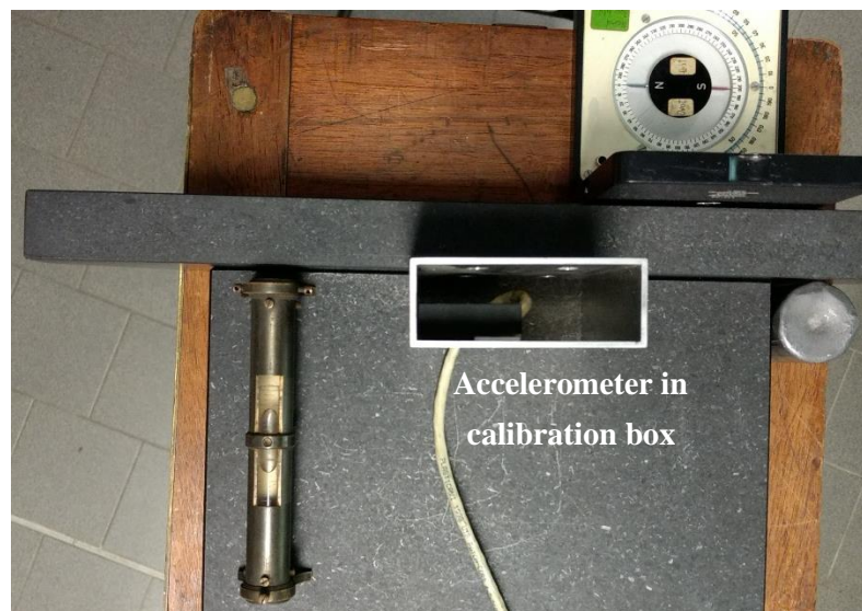
Figure 4. The accelerometer inside a calibration box during the six-faces test.
