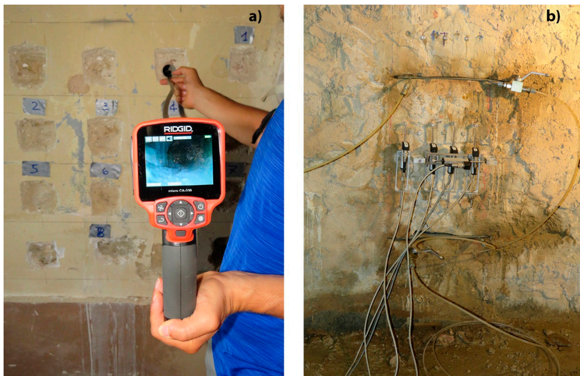
Figure 4. (a) Endoscopy test performed in the same area of the sonic test; (b) Double flat jacks test.
