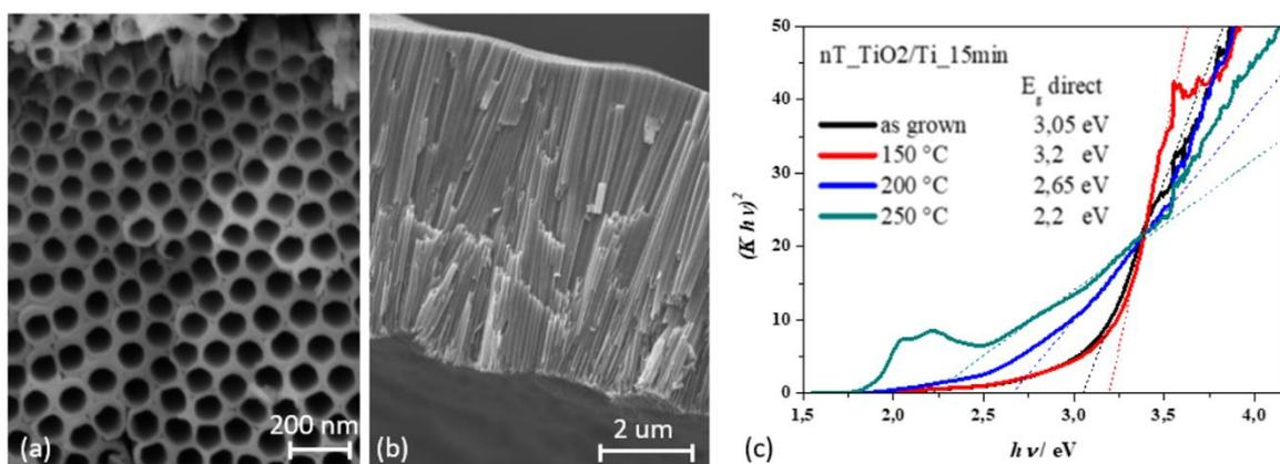
**Figure 3:** FESEM (a) top view and (b) cross view, (c) UV-VIS curves of the amorphous TiO<sub>2</sub> NTs.
