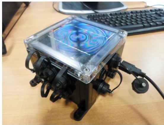
Figure 1. The Wasp mote with the embedded accelerometer used in the experiments.
