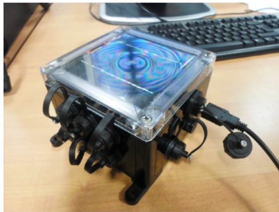
Figure 1. The Waspote with the embedded accelerometer used in the experiments.
