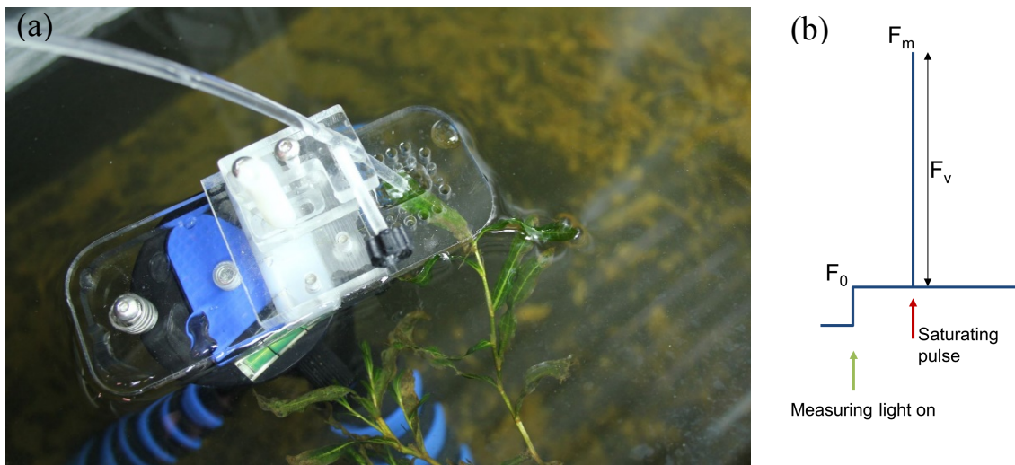
Fig. 2 (a) Details of a chlorophyll fluorometer: light pipe extension, leaf clip, and sampled leaf; (b) idealized chlorophyll fluorescence signal of a F_v/F_m test on a dark-adapted sample.
