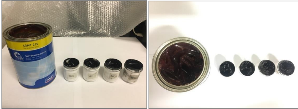
Figure 3.12. The five compounds of grease and graphene used for the tests.
