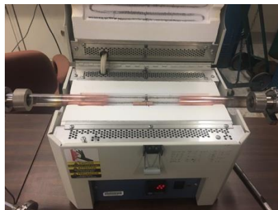
Figure 4.1. LPCVD furnace; example with copper samples inside.
