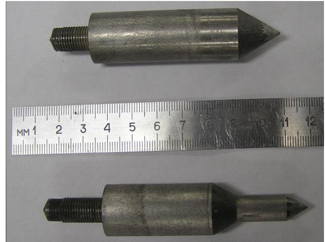
Fig.2. The heads of measuring bars used in the inverse experiments.
