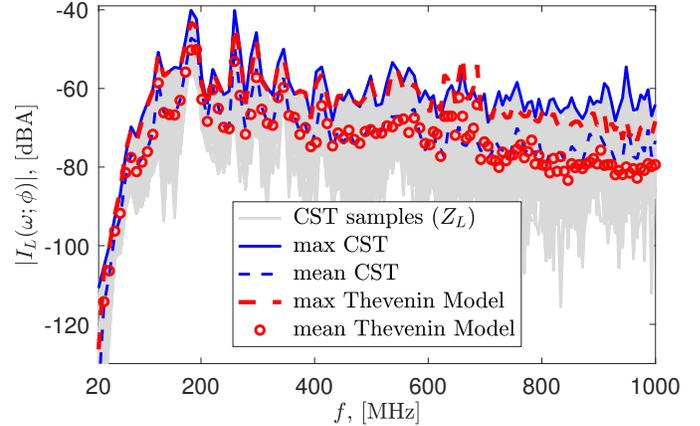
Figure 4: Magnitudes of the current induced in the ECU termination for 150 different incidence angles  $\phi$  (gray curves). The maximum and the mean values of the currents obtained via CST (blue curves and circles) are compared with the maximum values predicted the corresponding metamodel built from  $N_\phi^4 = 32$  samples (red curve and circles).
