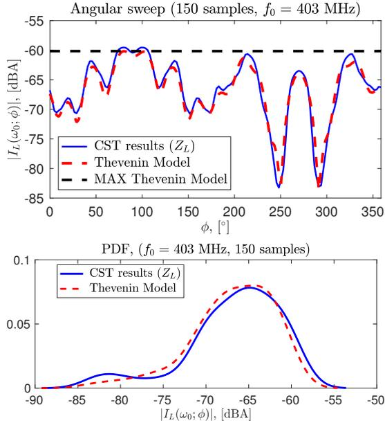
Figure 3: Induced current on the ECU termination for an incidence field at  $f_0 = 403$  MHz as a function of the angle  $\phi$  (top panel) and corresponding PDF (bottom panel), obtained via CST simulations (blue curves) and via the proposed modeling scheme with  $N_\phi^4 = 32$  samples (red curves).
