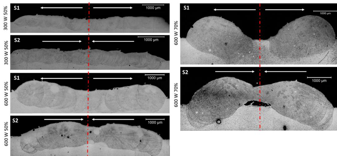
Figure 6. Optical micrographs of circular overlap samples.
