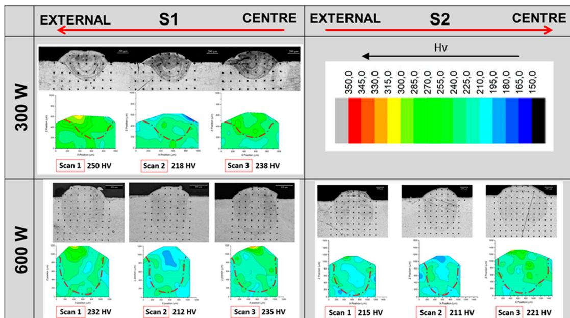
Figure 7. Micro Vickers maps: Circular contour samples.
