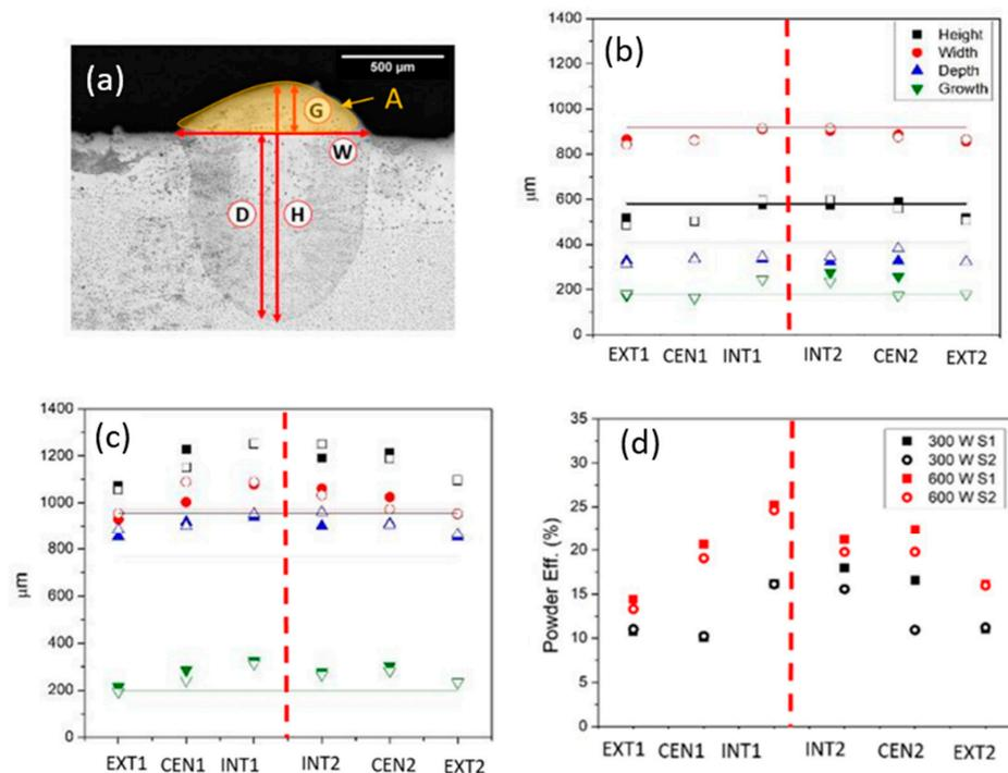
**Figure 5.** (a) Schematic representation of a metal bead with the geometrical features, (b) geometrical features of circular contour samples realised with (b) 300 W and (c) 600 W (S1 solid and S2 open symbols). Continuous lines represent the geometrical feature of the single scan track obtained with the same parameters. (d) Powder efficiency ( $P_e$ ) of circular contour melt pool.
