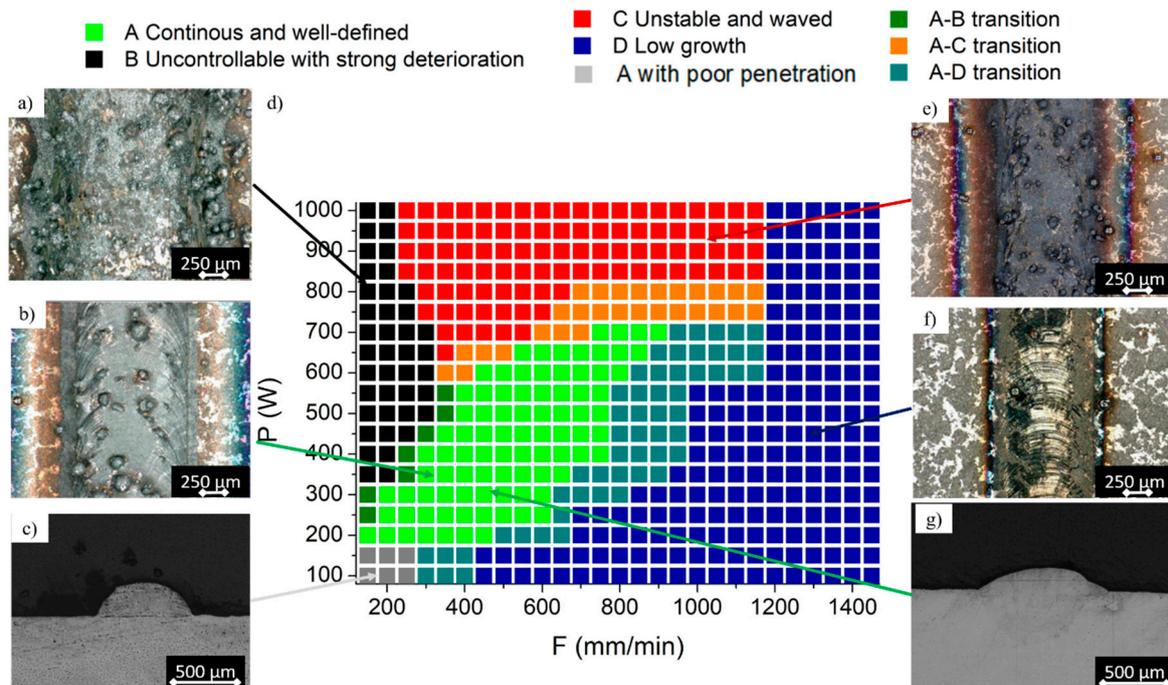
Figure 3. AISI 316L process parameter window through single tracks classification.
