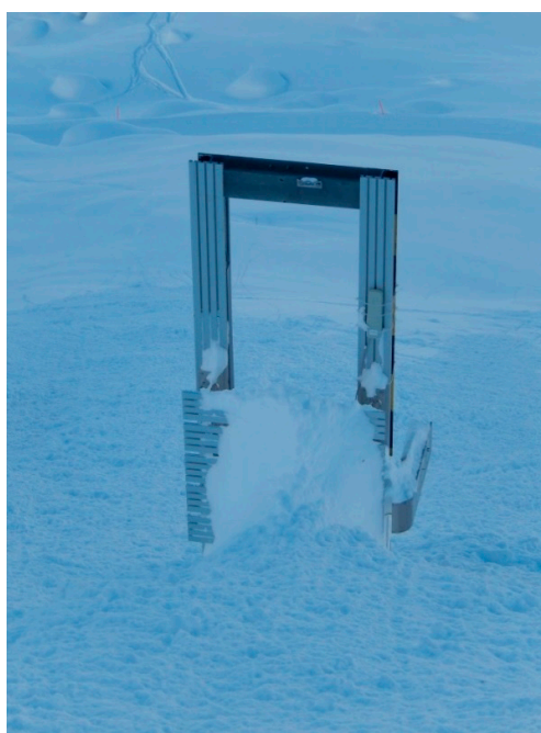
Figure 11. Deposition upstream the obstacle left from the avalanche on 20 January 2014. Photo E. Bovet.
