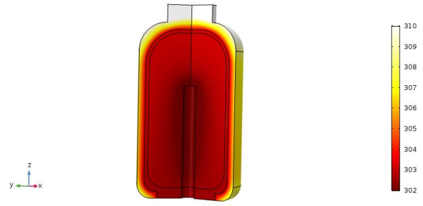
Fig. 25: Temperature distribution [K] in the Oxygen tank with 0.450 W.
