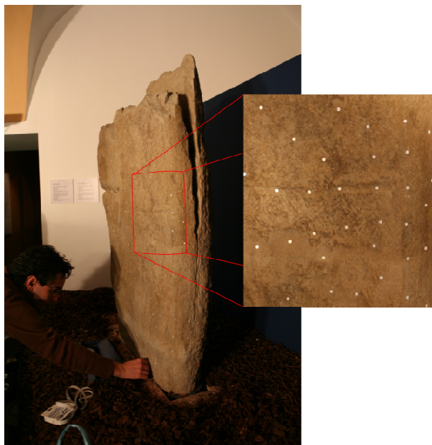
Figure 5. Placing the reflective targets on the object
