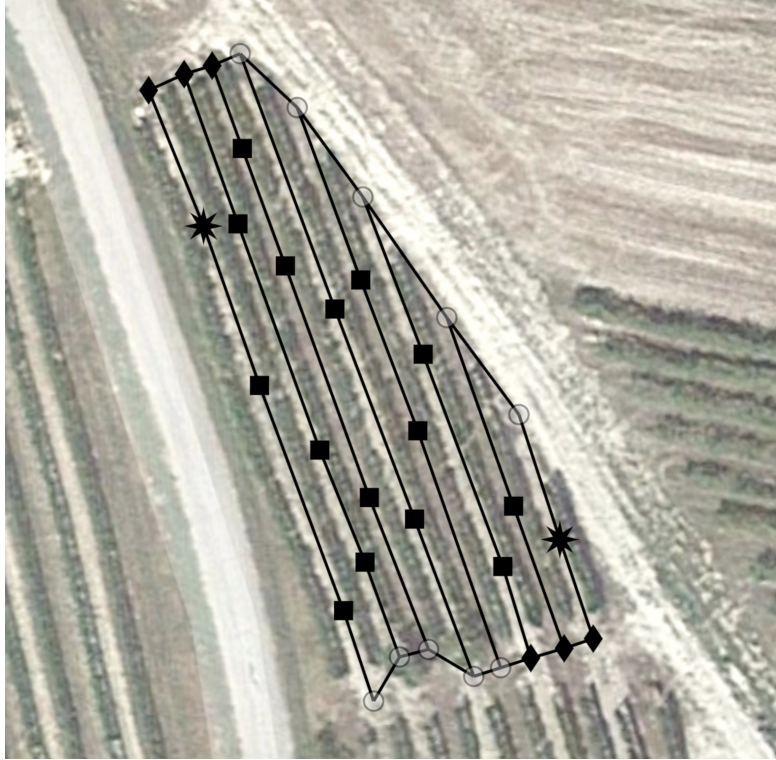
Figure 4: Undirected graph that represents the available paths for the UGV on a real vineyard. Nodes are marked as described in Fig. 3 and represent the type A, B, AB nodes with the addition of some “transit” nodes marked as empty circles.
