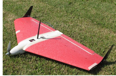
Fig. 1: The MicroHawk MH850 FW-UAV (credit:MAVTech).
