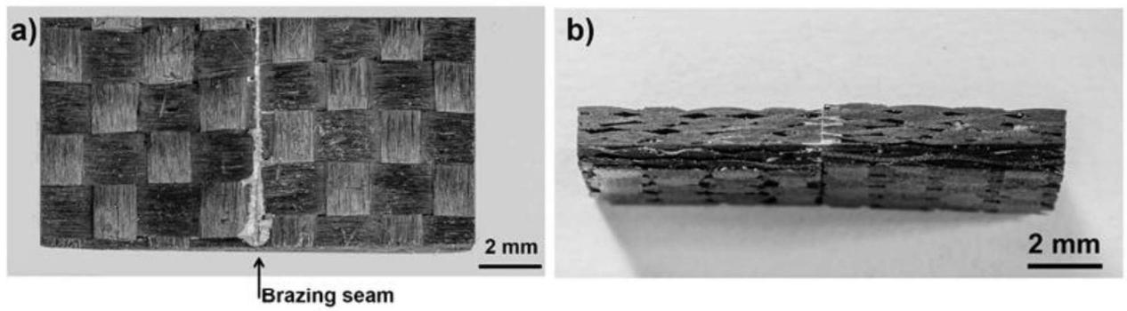
**Fig. 2.** Macrographs of an  $\text{SiC}_f/\text{SiC}$  to  $\text{SiC}_f/\text{SiC}$  joint obtained by means of AgCuTi : the braze seam is visible (a), as is the infiltration of the braze into the facing composite blocks (b); good adhesion and wetting of the filler alloy along the interface with infiltration of the alloy into the holes and gaps of the composites are visible.
