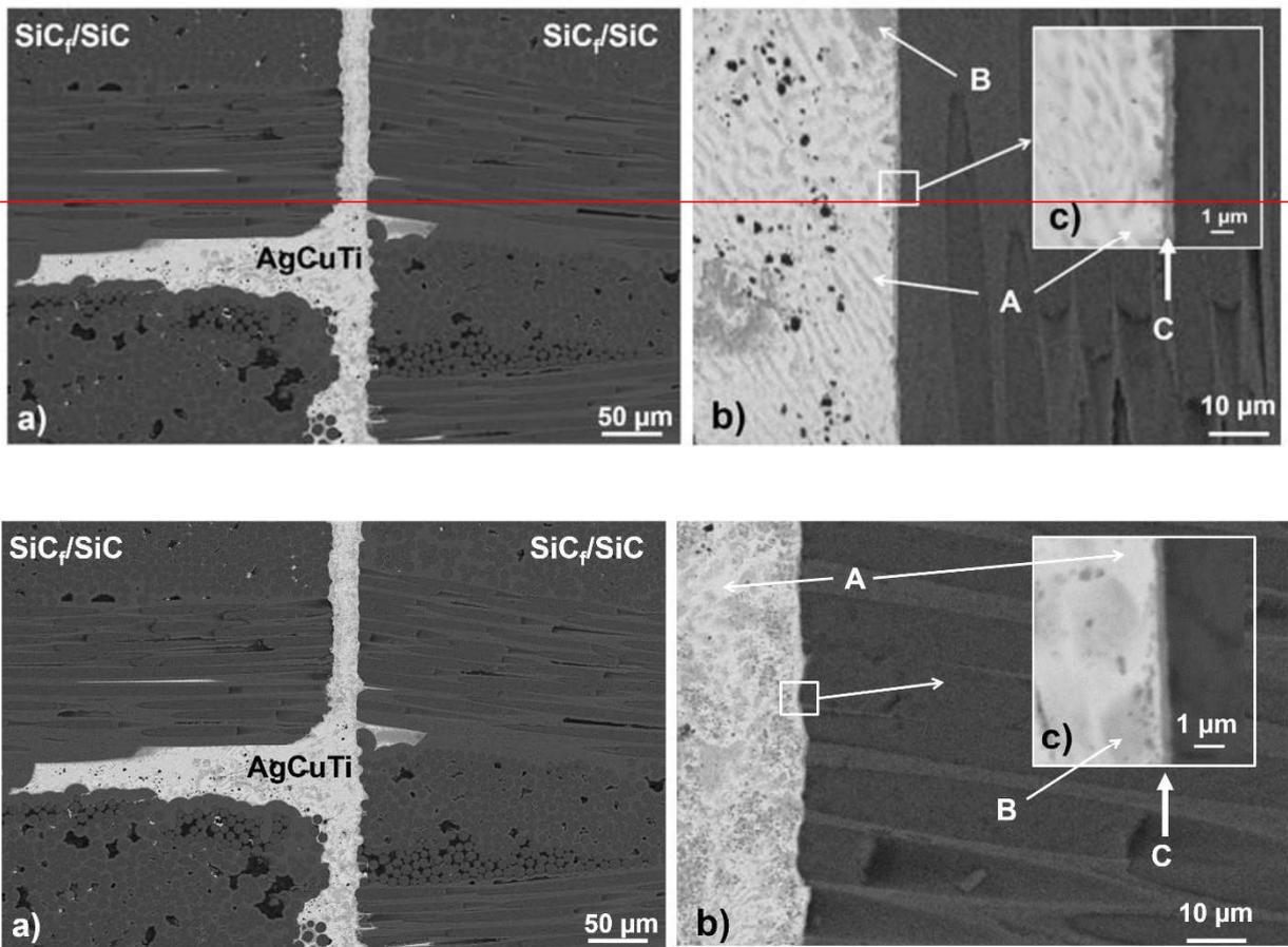
**Fig. 3.** SEM magnification of the cross section of an SiC<sub>f</sub>/SiC joint (as-received composite) showing: a) a panoramic view of the brazing seam showing infiltration into the composite porosities; b) adhesion of the brazing alloy at a microscale and c) higher magnification of the interface.
