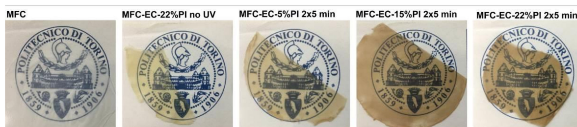
Figure 2. Photos of dry MFC mat, MFC-EC-22%PI composite before irradiation, and of composites irradiated for 2 × 5 min: MFC-EC-5%PI, MFC-EC-15%PI and MFC-EC-22%PI.
