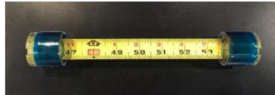
Fig. 2. Commercial tape spring; 170 mm sample
