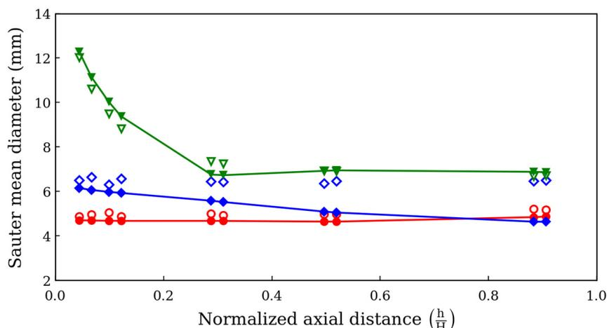
Figure 3: Axial profiles of the surface-averaged  $d_{32}$  obtained by PBM (solid line + marker) compared with the experimental measurements (hollow marker); red colour (Case 1):  $U_L, U_G=0.641, 0.0096(m/s)$ ; blue colour (Case 2):  $U_L, U_G=1.017, 0.0235(m/s)$ ; green colour (Case 3):  $U_L, U_G=0.405, 0.0368(m/s)$
