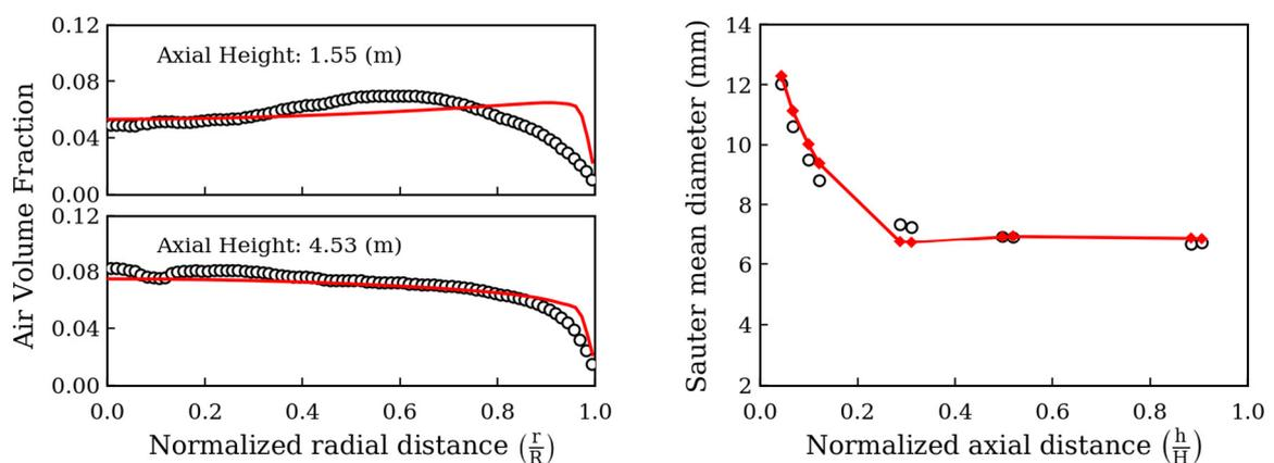
**Figure 1.** The radial profiles of the air volume fraction at two axial heights (left) and the axial profile of the average SMD (right) predicted by the two-fluid approach. Experimental measurements are shown by the circular markers.
