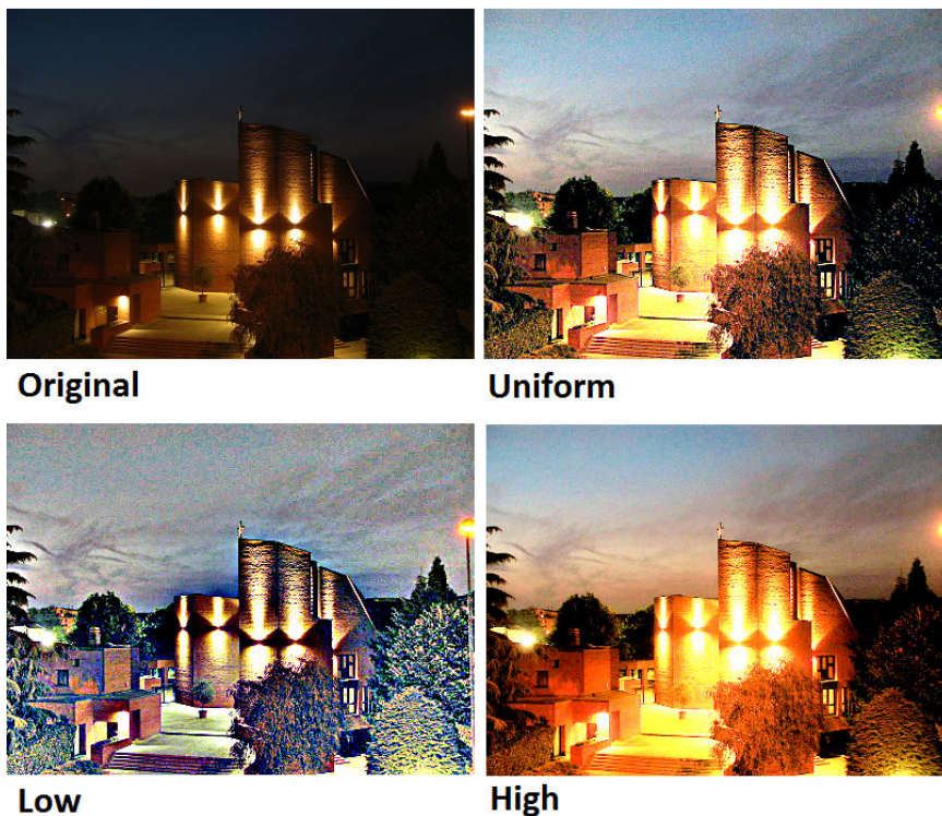
Figure 2: The original image is given in the left-upper panel, (Courtesy: Melari, Wikipedia, Curchby night in Monza). The other images had been obtained using GIMP Retinex at uniform, low and high levels. As in the Figure 1, the best level seems to be the low one.
