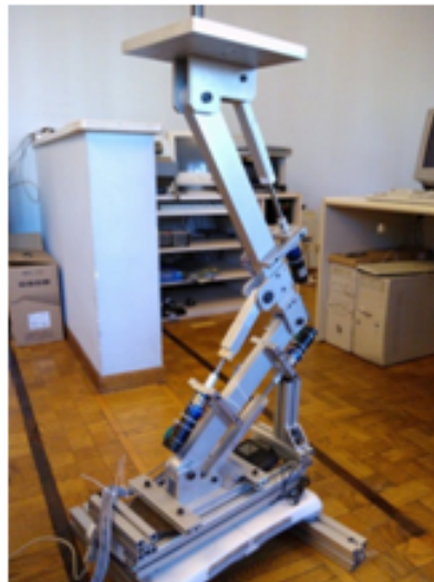
Figure 8. A small-scale 3 degrees of freedom (DOF) leg of the exoskeleton.
