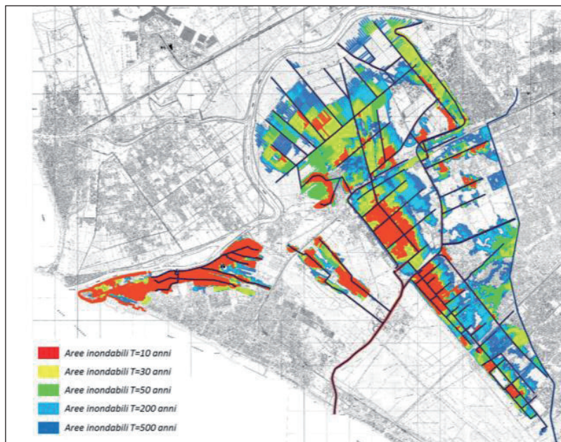
FIG. 1 X Municipio, Roma: Studio per il risanamento idraulico, estratto da Report RomaTre 10 th Municipality, Rome: analysis for hydrological renovation, from RomaTre Report
