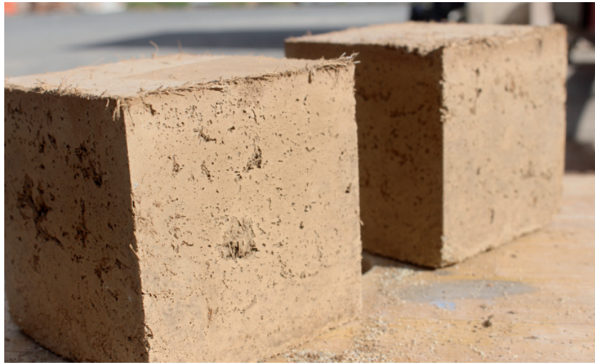
FIG. 1 Composito terra cruda e sisal Composite made of raw earth and sisal
