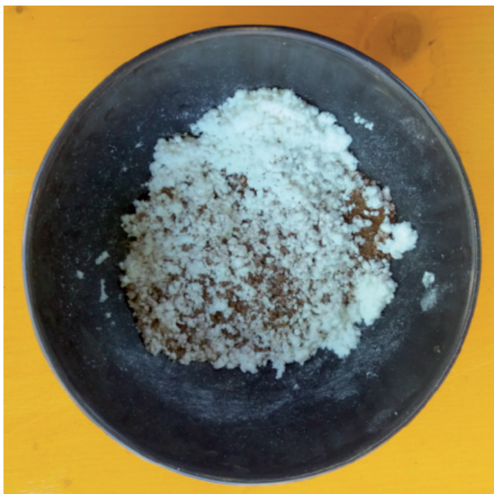
FIG. 1 Mix terra e cellulosa, rapporto 1:1 Earth and cellulose mix, ratio 1:1
