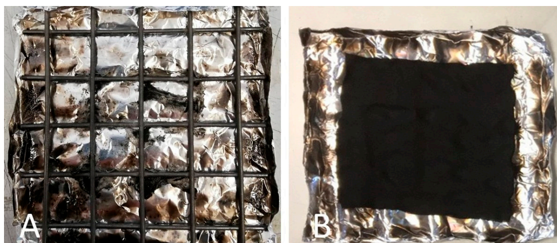
Figure 11. Residues of COT (A) and COT + SOL (70/30) (B) after cone calorimetry tests.
