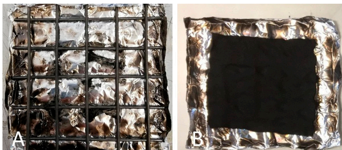
Figure 11. Residues of COT (A) and COT + SOL (70/30) (B) after cone calorimetry tests.
