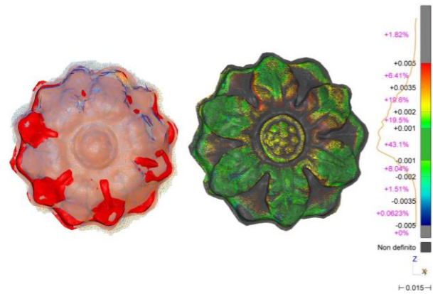
Figure 10. Comparison between the meshes of F6 medium range (yellow) and F6 short range (red).
