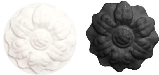
Figure 19. Printed object obtained with the described settings, white version for the test and black for the door integration.
