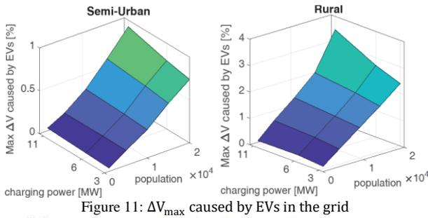
Figure 11:  $\Delta V_{\max}$  caused by EVs in the grid
