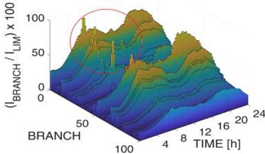
Figure 12: branch loading spatio-temporal distribution in rural network
