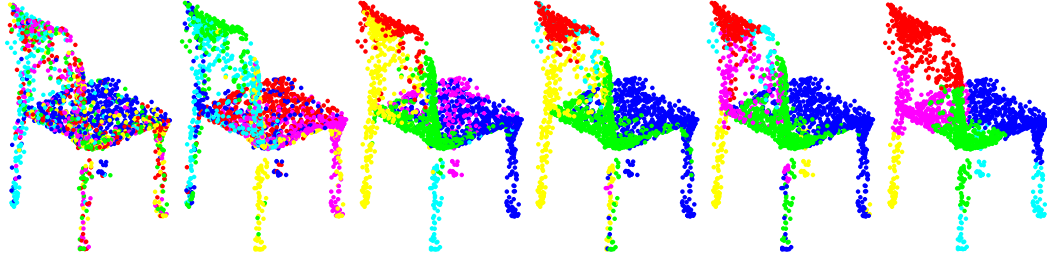
Figure 6: No upsampling: k -means clustering of features of intermediate layers, highlighted onto the output point cloud (leftmost: output of dense layer, rightmost: output point cloud). Notice how layer features generate clusters that are progressively more localized in the output geometry.
