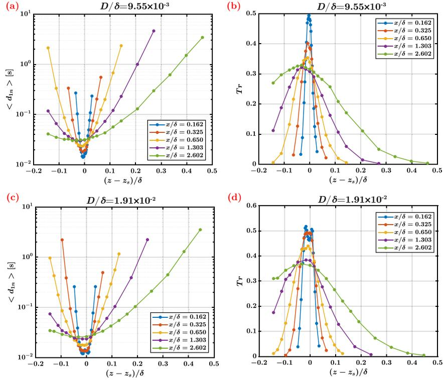
**Fig. 2** Network metrics as a function of the normalized wall-normal coordinate  $(z - z_s)/\delta$ , for different streamwise locations,  $x$ . Mean link-length (a) and transitivity (b) when  $D/\delta = 9.55 \times 10^{-3}$ . Mean link-length (c) and transitivity (d) when  $D/\delta = 1.91 \times 10^{-2}$ .
