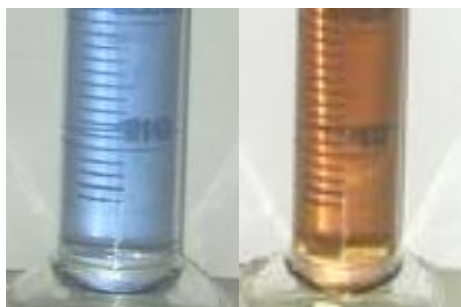
Figure 4. Water samples treated by Zincon: 1 ppm Zn (II), Zincon metal-chelated (left) and pure distilled water, Zincon free form (right).
