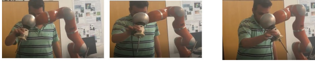
FIGURE 10. Hands-on motion of robot for data collection of orientation angles and force sensor measurement in free motion.
