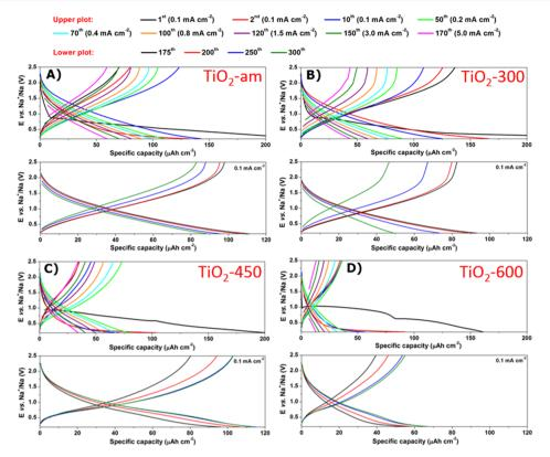
Figure 4. Ambient temperature electrochemical behavior of the different  $TiO_2$  NTs arrays under study:  $TiO_2$ -am (A),  $TiO_2$ -300 (B),  $TiO_2$ -450 (C), and  $TiO_2$ -600 (D). In particular, constant-current discharge/charge potential vs specific capacity profiles are shown between cycles 1 and 170 at different current densities from 0.1 to 5 mA cm<sup>-2</sup> (upper plots in A–D) and between cycles 170 and 300 at fixed 0.1 mA cm<sup>-2</sup> (lower plots in A–D).
