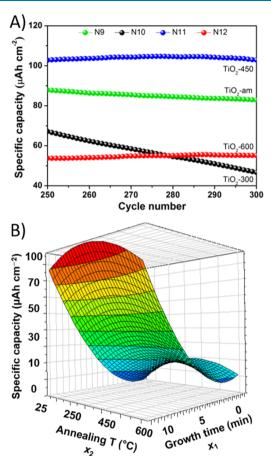
**Figure 6.** (A) Specific discharge capacity values under  $0.1 \text{ mA cm}^{-2}$  for sodium cells assembled with  $\text{TiO}_2$  NTs array working electrodes (growth time = 10 min) between the 250th and 300th cycle; (B) response surface showing the effect of annealing temperature and growth time on the specific capacity at the 250th cycle of lab-scale sodium cells.
