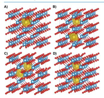
**Figure 8.** Structural models for a second  $\mathrm{Na}^+$  cation placed in different configurations: (A) as next-neighbor along the same [001] channel; (B) in the furthest position within the 96-atom supercell; (C) in an adjacent site of a parallel [001] channel; (D) in a parallel [001] channel bridged by a  $\mathrm{TiO}_6$  moiety: the central  $\mathrm{Ti}$  of such moiety strongly goes off-center upon relaxation. Color code as in Figure 7.
