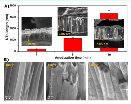
Figure 2. (A) Graph of TiO<sub>2</sub> NTs length vs time of anodization; FESEM images showing different NT lengths are shown as insets. (B) High-magnification FESEM images of the NTs annealed at different temperatures, namely 300, 450, and 600 °C, for 1 h in ambient atmosphere.
