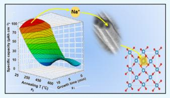
allows identifying anatase at high growth time as the TiO2 polymorph of choice as an anode material, thus creating a benchmark for sodium-ion batteries, which currently took the center stage of the research in the field of energy storage systems from renewables.
