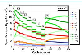
**Figure 3.** Specific discharge capacity vs cycle number at different current densities (from 0.1 to 5 mA cm $^{-2}$ ) for sodium cells assembled with  ${\rm TiO_2~NT~arrays}$  as working electrodes, as described in Table 1.
