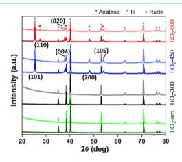
**Figure 1.** XRD patterns of  ${\rm TiO_2}$  NTs nonthermally treated and thermally treated at 300, 450, and 600 °C. Dark colors indicate samples before cycling, while light colors refer to cycled electrodes. The growth time by anodic oxidation is kept constant at 5 min.
